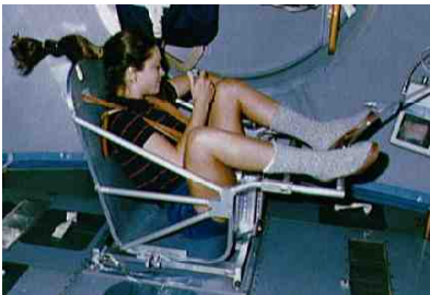
g / Astronaut Tamara Jernigan measures her mass aboard the Space Shuttle. She is strapped into a chair attached to a spring, like the mass in figure f. (NASA)
